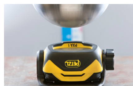
Impact resistance test
